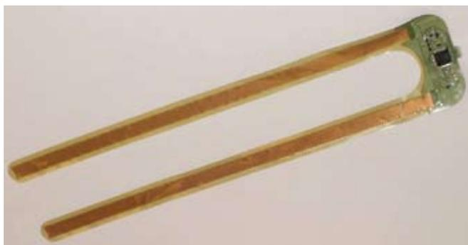
Figure 11: Integrated stretchable Ruler in SCB design
