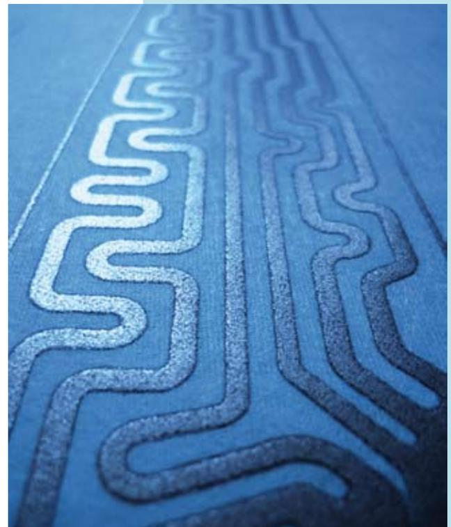
Figure 1: Conductive Paste on Nonwoven
