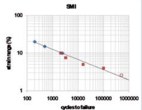
Figure 4: Cycles to failure of the SMI technology for different stretch rates
