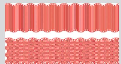
Figure 10: One side meandered capacitor plates & two directional meandered capacitor plates.
