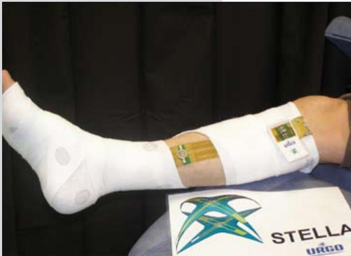
Figure 2: Urgo band aid demonstrator for pressure measurement under compression garments.
