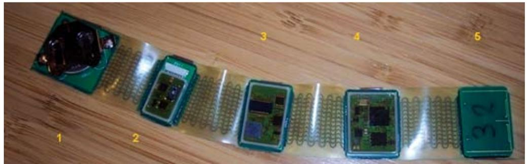
Figure 6: Activity monitor hardware in SCB technology partitioning (from left to right): Battery (1), power management (2), sensor board with 3D accelerometer and 2D magnetometer (3), microprocessor (4) and 2.4 GHz radio with antenna on top (5)
