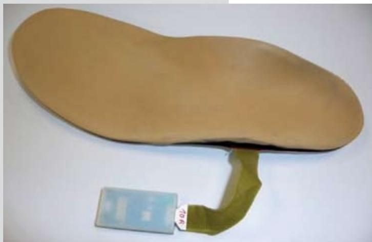
Figure 7: Shoe insole demonstrator in SCB technology
