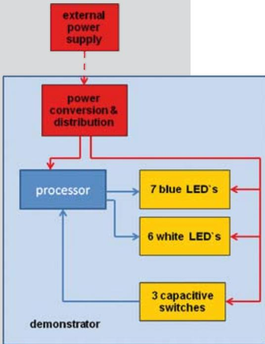
Figure 12: New sensor node architecture
